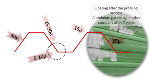
Coating after the profiling process – eg. powder coating: separation of paint because of cracks caused by uneven coating on bends.
