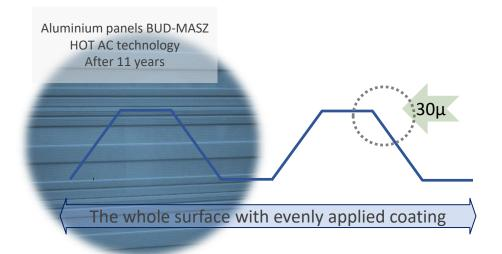
Coating before the profiling process— even coating on both sides. BUD-MASZ HOT AC technology.
